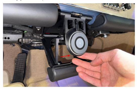
• When closing, press the magnet holder back in slightly and then fold up the knee protection cover until the holder snaps into place at the top
